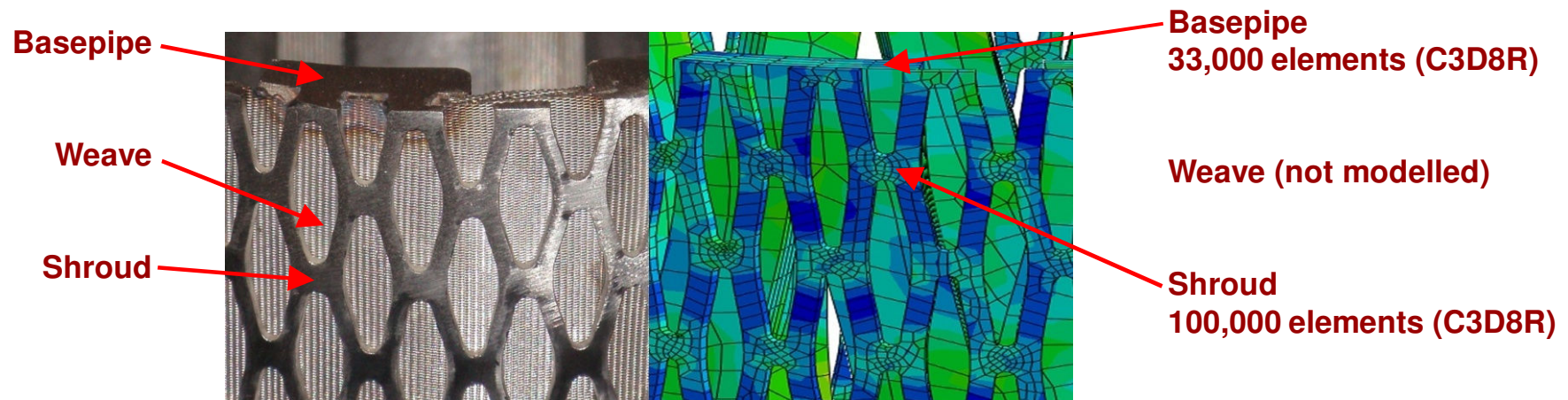
Detail of ESS construction showing complexity of the meshing on the shroud
