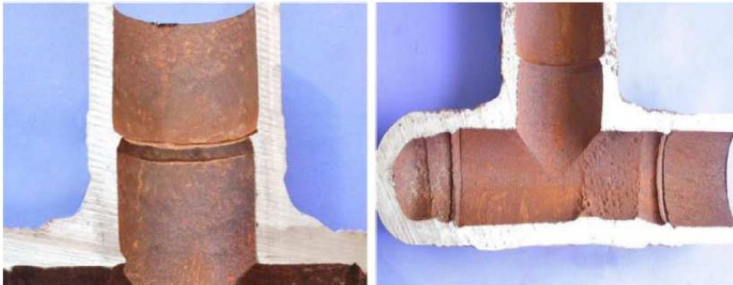
Figure 1: Indication of weld and flow-induced corrosion from metallurgical analysis KA 15 flowline.
