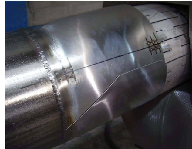
Model #10 During fabrication – with circumferential weld
