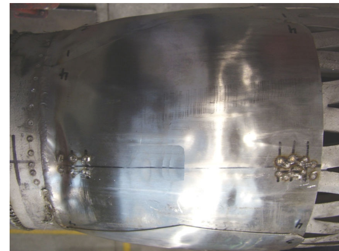
An expanded example (shroud and filter layers stripped off)
