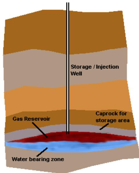
Figure 3 depleted gas reservoir UGS
