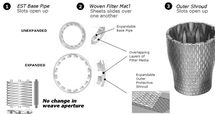
**Figure 1 Details of the Construction of ESS**
