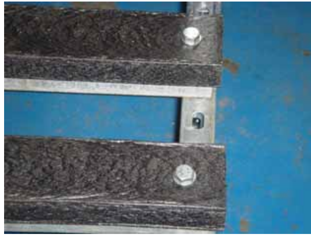
M12 bolts were used to secure the plastic to the unistrut
